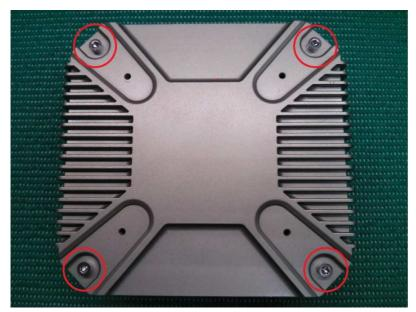
**17.)** Insert the cover screws and secure in the order of opposite corners (diagonally) to ensure even pressure.
