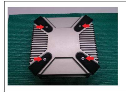
**1.)** Unscrew the 8x screws (4 top, 4 bottom) to remove the rubber feet.
