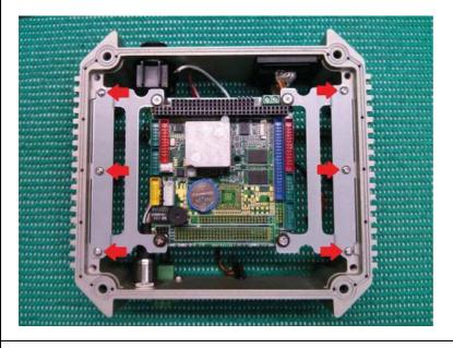
**13.)** Place the VSX-6150E-V2/bracket assembly back into the chassis and secure with the 6x screws.
