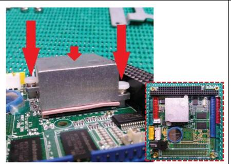
**9.)** Align the aluminum heat sink according to the nylon pin holes located on the unit and place on top of the heat conductive pad.
