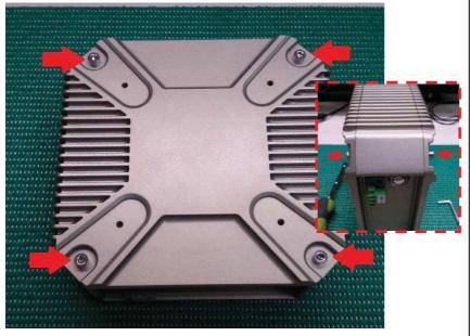
**2.)** Using a 5/32 allen wrench and a 5/16 socket wrench, remove the 4x cover screws.
