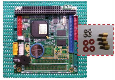
**5.)** Prepare the following materials for mounting the standoffs onto the VSX-6150E-V2.
