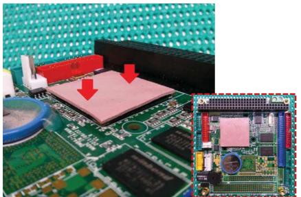
**8.)** To mount the heat sink, place the heat conductive pad on top of the CPU.
