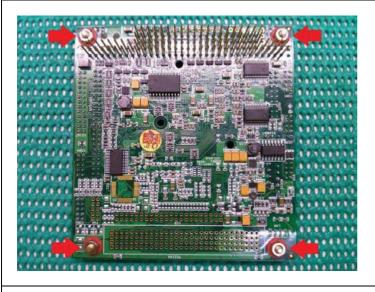
7.) Insert a washer and nut onto the standoff from the bottom of the unit and securely tighten.
