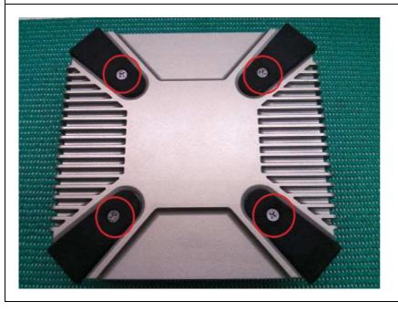
**18.)** Reinstall the rubber feet onto the chassis and securely tighten the screws.
