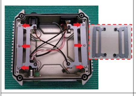
**4.)** Unscrew the 6x screws to remove the PCB bracket.
