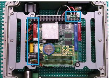
**14.)** Plug in the cables accordingly.
