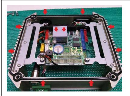
**15.)** Place another heat conductive pad on top of the heat sink.
