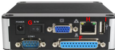
F: Printer port G: Power Switch H: 10/100 Mbps LAN I: USB
